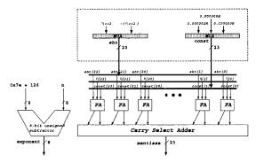
Fig. 7. Exponentiation approximation unit. An 8-bit subtracter is used to make the exponent part and a 23-bit CSA is used to make the fractional part.
